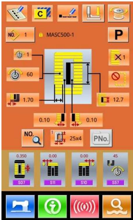
In the Mode Setting Level 2 interface, press
