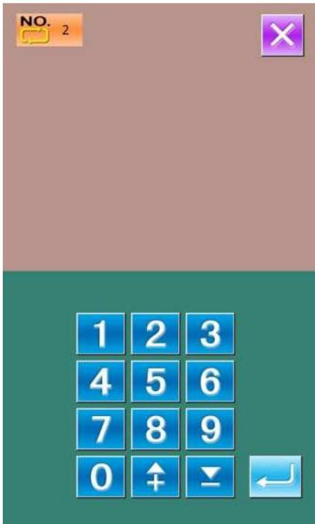
Press the new pattern registration key
