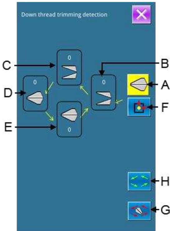
In the interface of Test Mode, press
