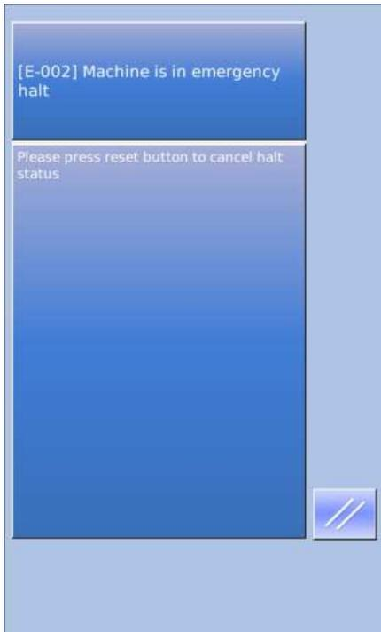
When STOP switch is pressed during sewing, the sewing machine interrupts sewing and stops. The interface, as the figure at right, is displayed
