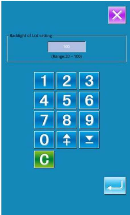
In the Mode Setting Level 2 interface, press
