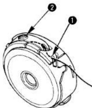
When the threading open ① is at up position, user need pull out the bobbin thread upward and adjust the tension in the way below:
