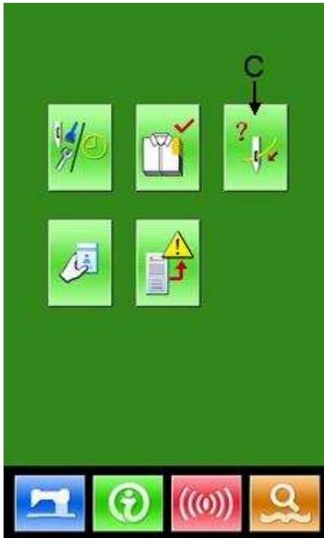
In information interface, press
