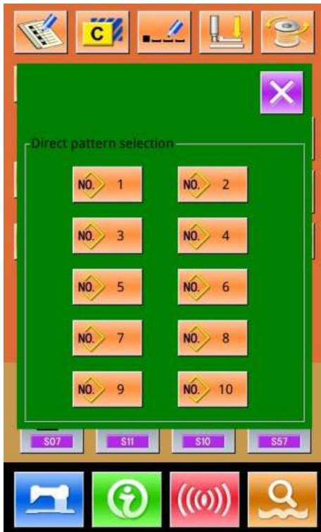
The user can register the 10 frequently used patterns to the direct keys for selecting directly, press
