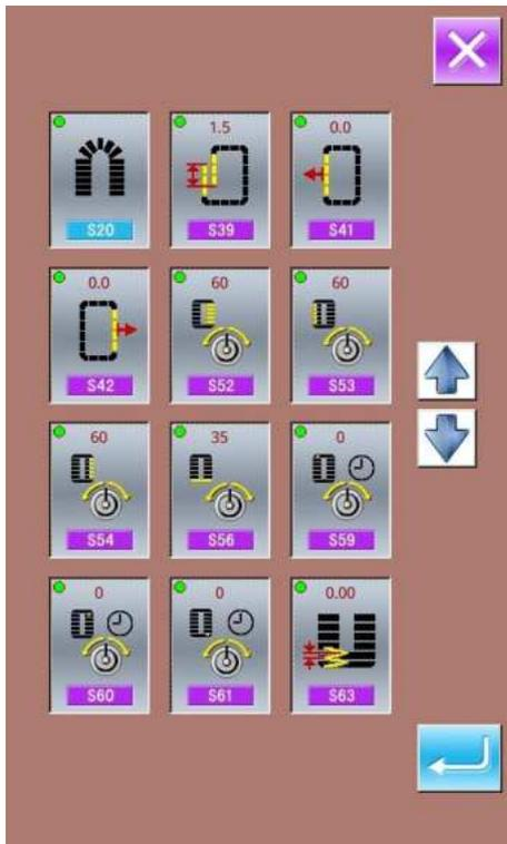
Some sewing data can be set to be opened, press
