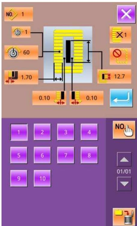
10 pattern numbers can be registered to the direct buttons at most. On 10 displayed direct buttons, the user presses the button he wishes to register, and then enters the pattern select interface. (as shown in the right figure)
